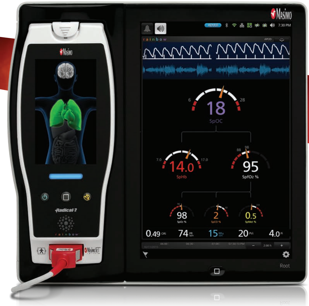
Utilizing more than seven wavelengths of light and breakthrough signal processing, Masimo’s rainbow® Pulse CO-Oximeters can measure and display oxygen content (SpOC), along with total hemoglobin concentration (SpHb) and fractional arterial oxygen saturation (SpfO2)
