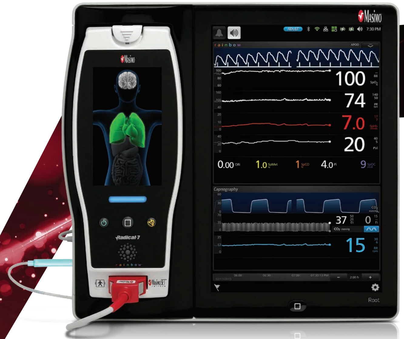
Capnography and Gas Monitoring are "plug and play" MOC-9 modules
